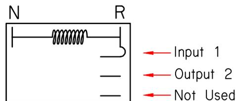
The above circuit is designed to automatically start the Vacuum Motor when any of the connected tools is powered on. Only two are shown but any number of additional tools may be added in the same way. Just repeat the circuit shown, in this case, for a Router.
