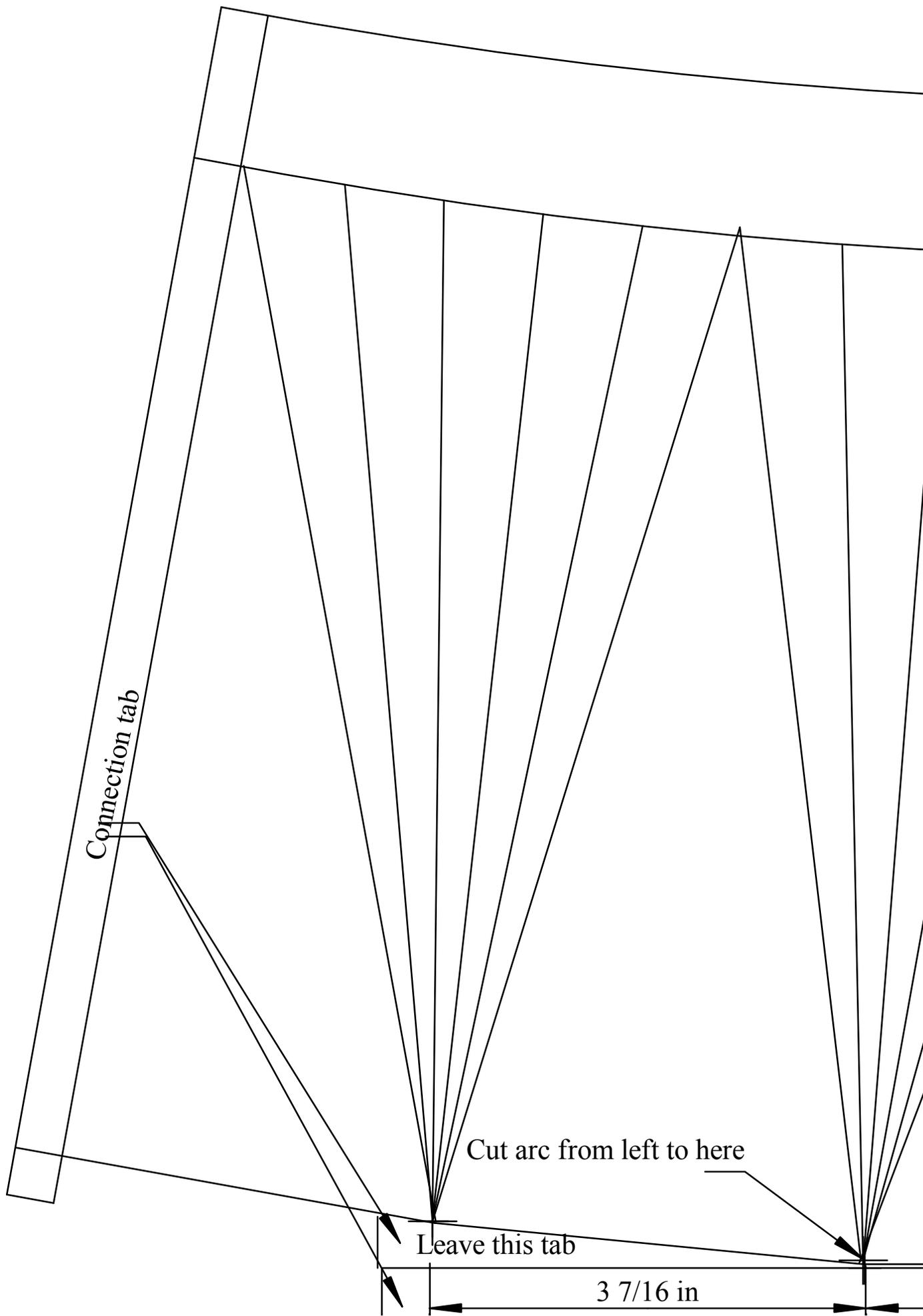
5 inch Round end extension for connecting finished adaptor
