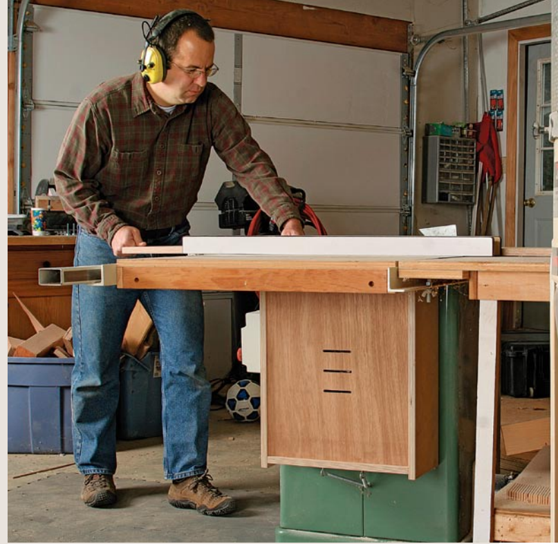
Add intake. Christiana had a plywood box covering the motor opening. So he just routed three slots, positioned to wash cool air over the motor.
